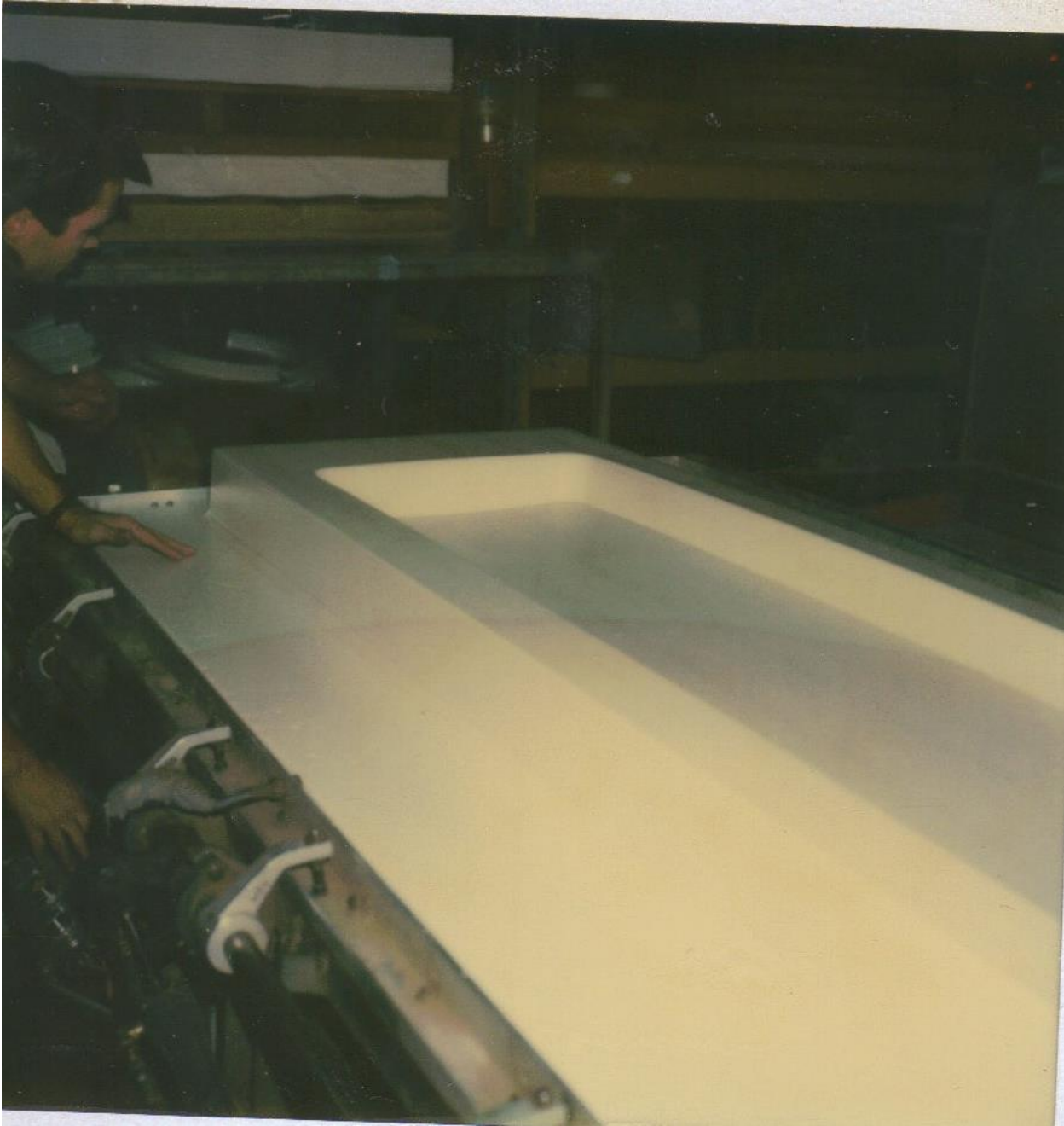
2'-0" shell part before trimming
