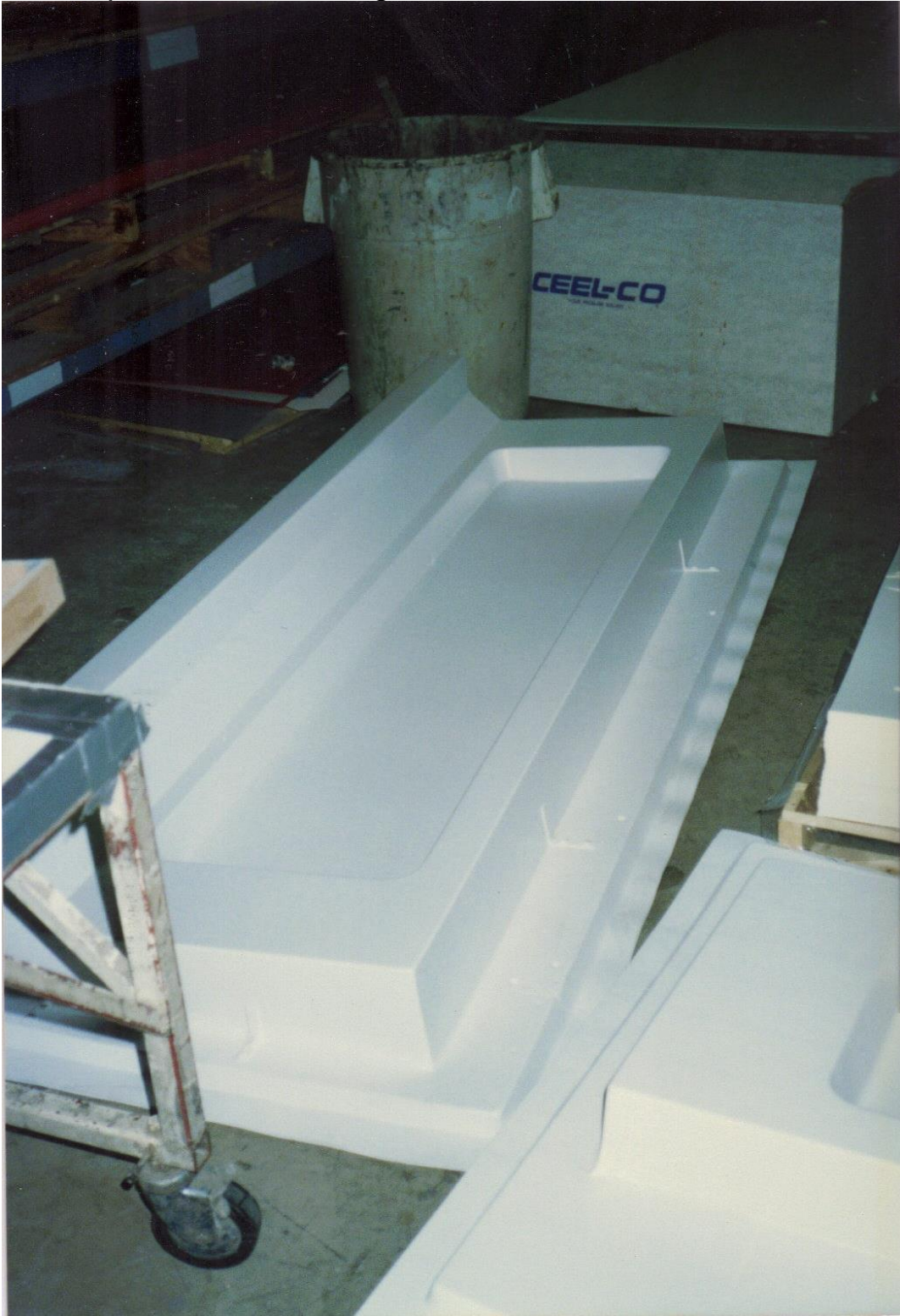
Corner part before trimming
